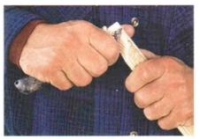
Beveling the back of a miter eases a tight fit. Back-beveling reduces friction when fitting and helps to ensure that the miter's face is tight.
