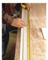
Using a square, the author will extend marks across all the stiles. The rails will butt these marks. Marking several members at once ensures consistent spacing.
