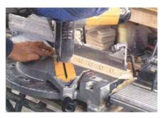
**Short pieces of molding are mitered to length using a stop block.** This production technique is reliable because the stiles were also cut using a stop block.
