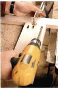
**Locking pliers clamp rail to stile.** Because of their low angle, pocket screws pull the joint together tightly with little movement of the pieces.
